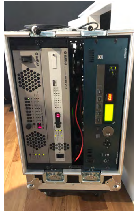
The Piano Centre's AFC3 processor racked up. Usually hidden in the cupboard, it can be wheeled out for maintenance
