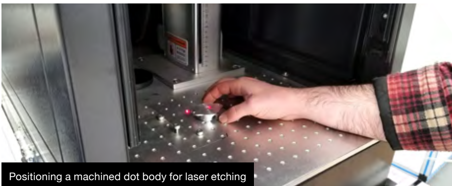
Freshly machined SmartPXL40 body
