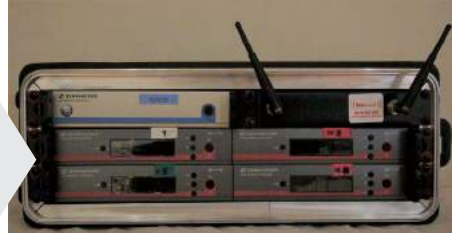
Sennheiser antenna splitter and receivers
