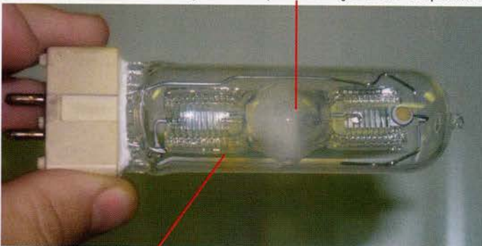
Yellow banding on external glass changes the colour temp of the light
