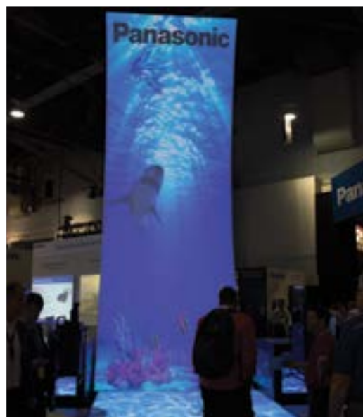
Panasonic shows off, edge blending four projectors to a curved screen
