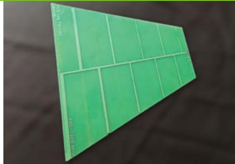
PCB Log Periodic Antenna Just solder on a connector and fit a mount and you have an excellent paddle. Can be painted without affecting performance.
