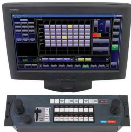
VINTEN RADAMEC CONTROL PANEL
