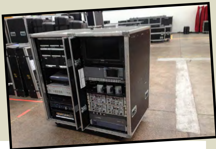
Left: 4 camera flyaway video camera system which includes a Sony DFS800 switcher, 4 Sony D50 Camera Control Units, a 40 x 40 Black Magic SDI Router, a Clearcom 36 port Matrix Comms Master, a Hamlet vectorscope, 2 clearcom V Panel intercom stations and enough monitors to function effectively.
