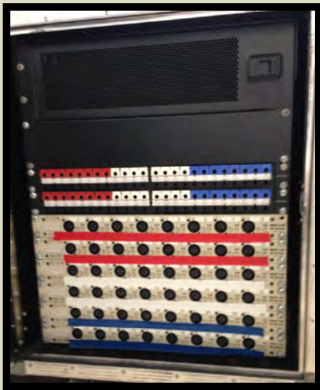
A 48 channel passive 3 way split with a patch bay at the input stage. It provides a direct, ground lifted and isolated output from stage inputs.
