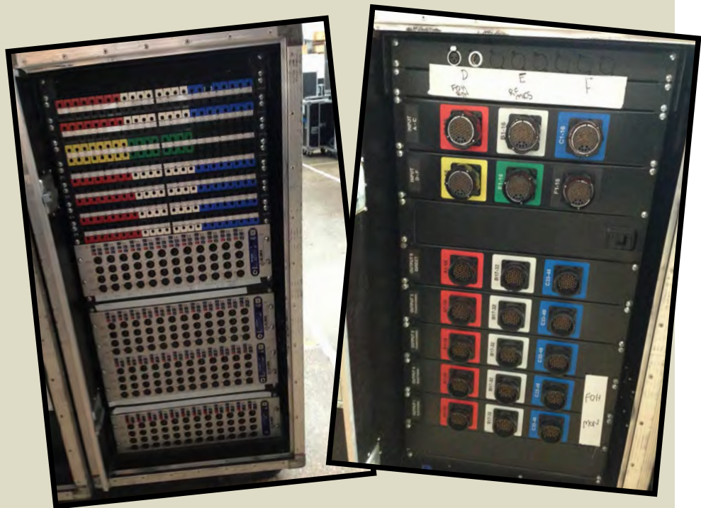
Above: Front and back of the 48ch active split system incorporating a long-frame patch bay. It essentially is a 5 way 48 channel split with the ability to route 96 input lines and 96 output via the patch bay making it very quick to access and patch in a special event environment.
