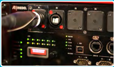
LIGHT-UP BNC CONNECTORS SHOW SIGNAL PRESENCE
