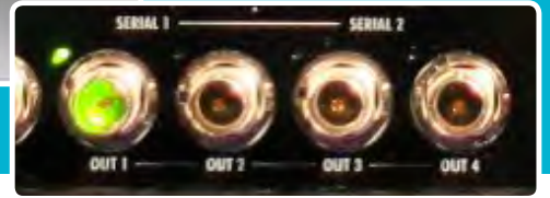
LIGHT-UP BNC CONNECTORS SHOW SIGNAL PRESENCE
