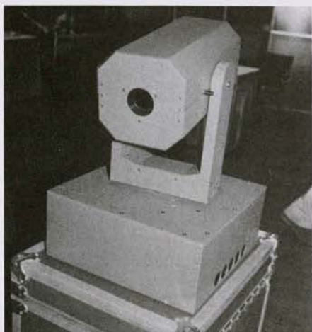
Taiwan copy of a VL-1 Vari*Lite. Note the stopper pin on the side, which prevents the creature from doing a loop the loop when the computer goes berko.
