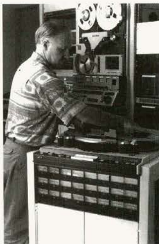
Tony Webb of Phoenix Audio with his new Otari 24 track MTR90 III
