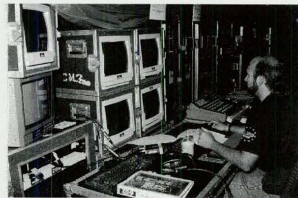
in the 'Underworld' - video control gear. The Digiwall and Vidiwalls are driven by Philips Digi!a! Image Controllers. (See story, next page for details).
