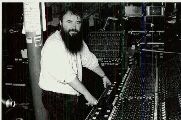
Joe O'Herlihy in work mode. The new ATI Paragon console with a noise gate and compressor on each channel is joined by the original Clair Bros. 'Classic' on Joe's left.
