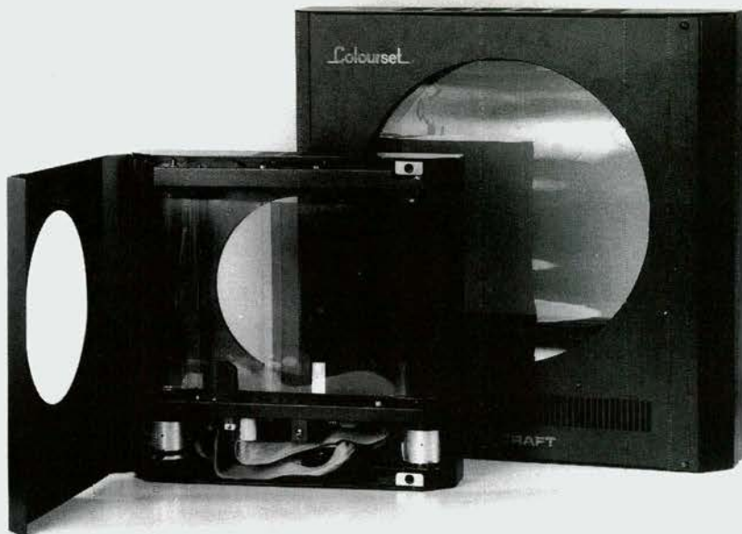
Colourset 1K (left, with its guts exposed) and 2K scrollers. The silver rectangle on the bottom edge of the 1K's gel scroll is a marker tape - the key to lining up each gel frame precisely even when it gets distorted. The infrared 'eye' (to the left of the tape in the picture) 'sees' each marker tape as it goes past and the unit's software tells the motors what to do.
