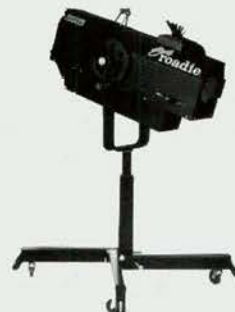
HTI 400 "Strong" Roadie Medium Throw 3.5-9° Built in colourchanger 1000 Lux @ 53 metres
