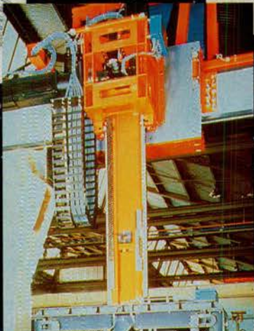
OLFLEX.FD-800 and FD 855P energy chain cable systems.
