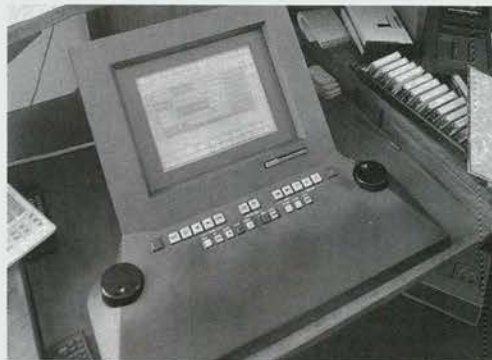
EDI-Tracker, a non-linear audio editing system developed by Soundfirm.
