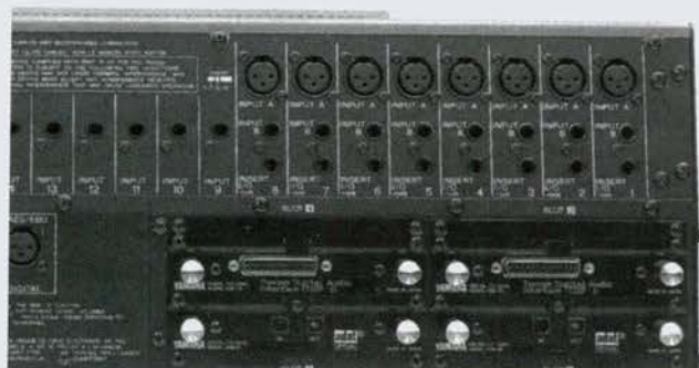
4 slots allow optional direct-digital to/from ADAT, DA-88 and others.
