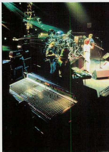
The PA People have further upgraded rental inventory with the addition of a new Soundcraft SM12 monitor console - it provides 12 foldback mixes, and has 48 inputs.
