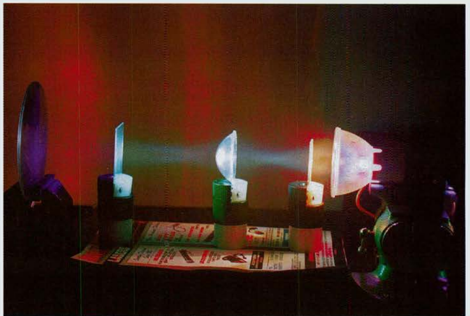
Optical Prototype. Early workbench tests of dichroic filters and metal halide light source used to develop optical configuration of first Vari*lite prototype.
