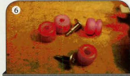
Save two of these silicon suspension grommets from the CD drive.
