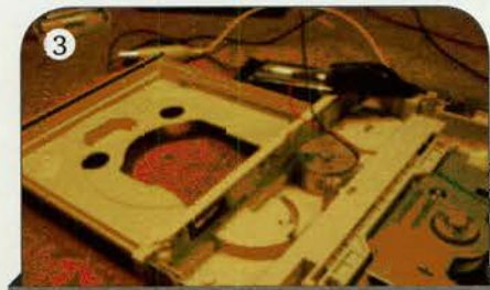
Power up the motor and get the drawer open.
