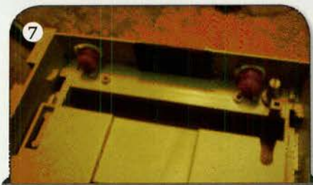
Use grommets as end stops so that the drawer rack doesn't disengage with the drive pinion.
