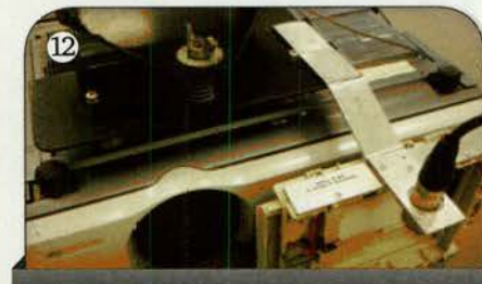
The finished shutter permanently mounted onto the projector bracket.
