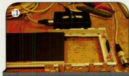
The shutter which weighs only 200g is ready for mounting on the projector bracket.
