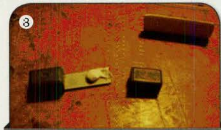
Crack the magnet out of its case and re-glue so that it has a lower profile for clearance.
