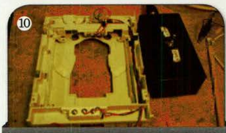
Play with the position of the 'open' reed switch to coax the maximum travel drawer travel.
