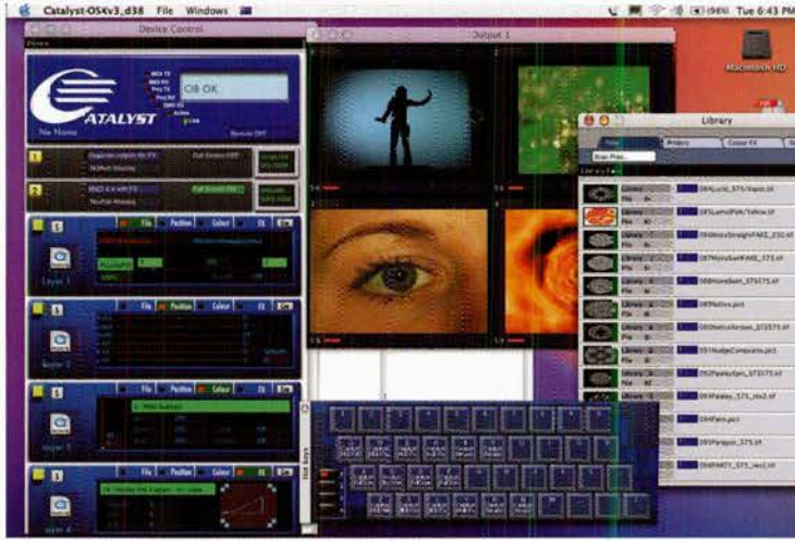
This screen image of the Catalyst system shows the four source and two output control panels on the left, the four window "layer preview" screen, the source file list and the Qwerty hot key set L3 panel.
