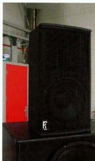
Alcon's approach uses the new ribbon high frequency device, and traditional cone drivers for mid and low frequencies.
