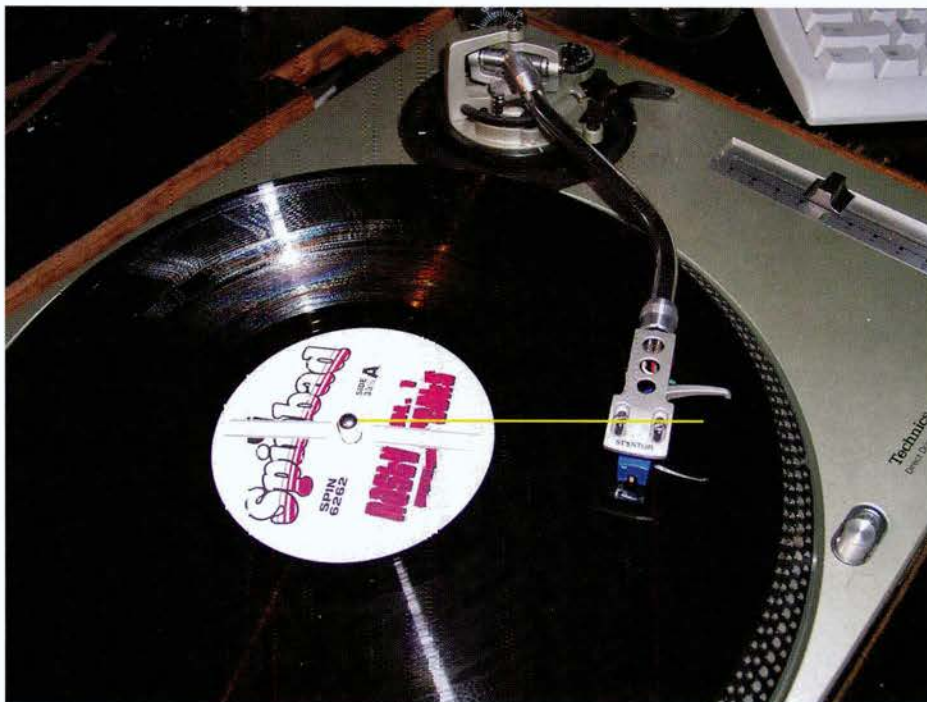
Styli out of alignment. The screws should bisect a line from the centre of the record when the arm is at middle. Like above.
