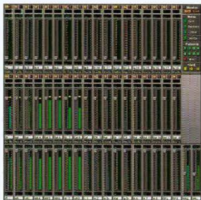
THE TOTALMIX SOFTWARE LETS YOU MONITOR AND ROUTE THE MULTIFACE'S AUDIO INS AND OUTS. THIS SHOWS FOUR STEREO PAIRS PLAYING OUT OF A BLEND OF LIVE, AND THROUGH THE HARDWARE CLTS.
