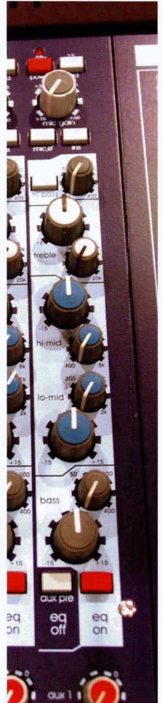
Whole lotta EQ (above). A Really cool idea: you can switch the EQ out of the auxiliary chain. Most excellent if using an auxiliary for stage monitors from the front of house console.
