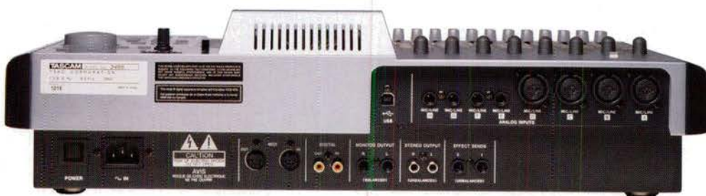
THE REAR PANEL I/O BELIES THE LOW PRICE; THERE'S USB 2.0, SEVERAL AUDIO OUTS, MIDI, AND EIGHT AUDIO INS.
