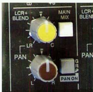
Main mix button selected, Pan selected and stereo pan is hard right, the LRC blend control is centred. All normal. We strongly suggest all engineers obtain a simple test tone generator (we use an NT Minirator, which does tones plus a lot more and etc) with any new console for a while, seeing where the signal goes, using the output displays. This part should be obvious - there is no need to have the rest of the system working - so you don't need to deafen yourself and start other people complaining about the wall of pink noise or the 1kHz tone!
