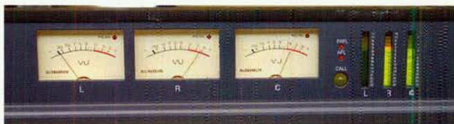
Main mix button selected, Pan selected and stereo pan is hard right, the LRC blend control is centred. All normal. We strongly suggest all engineers obtain a simple test tone generator (we use an NT Minirator, which does tones plus a lot more and etc) with any new console for a while, seeing where the signal goes, using the output displays. This part should be obvious - there is no need to have the rest of the system working - so you don't need to deafen yourself and start other people complaining about the wall of pink noise or the 1kHz tone!
