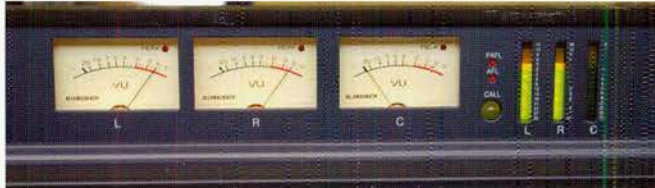
Main mix button selected, Pan selected, but the LRC blend control is swung hard left. Centre signal now absent. Predictable.
