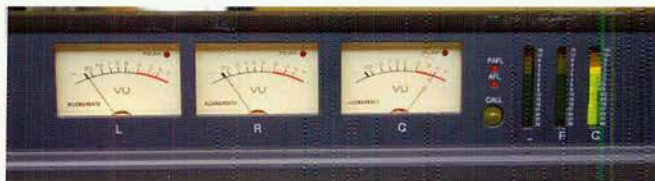
Main mix button selected, Pan selected, but the LRC blend control is swung hard right. Centre signal now is the only output. Also predictable.
