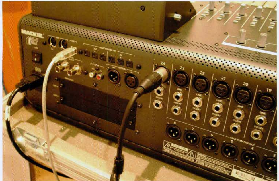
Out back, way heaps of connectivity, straight out of the box. Expansion slots make a way to connect two consoles together, for 26 facers. Adat Lightpipe in means 24 digital inputs for your 3 x external 8 channel analogue to digital converter boxes.
