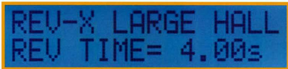
THE LCD CHANGES COLOR TO INDICATE THE TYPE OF EFFECT BEING USED.
