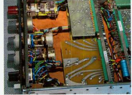
FIG. 3. THE IDENTICAL TRACES ARE ATTRIBUTABLE TO USING THE ORIGINAL PCB ARTWORK FROM THE NEVE ARCHIVES. NEW (LEFT) AND OLD (RIGHT).
