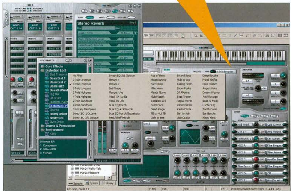
THE PATCHMIX DSP APPLICATION (LEFT) PROVIDES 32 CHANNELS OF ZERO-LATENCY HARDWARE MIXING/MONITORING, AND A VIRTUAL PATCH BAY WITH FX INSERTS. IN THE BACKGROUND IS THE EMULATOR X'S VOICE EDITING WINDOW, WITH ONE OF THE 54 FILTER TYPES ABOUT TO BE SELECTED.
