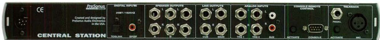
CENTRAL STATION FEATURES RCA AND BALANCED 1/4" ANALOG INPUTS. NOTE THE XLR TALKBACK MICROPHONE INPUT, WHICH ALLOWS YOU TO USE YOUR OWN MICROPHONE IN PLACE OF THE CENTRAL STATION'S BUILT-IN MIC.
