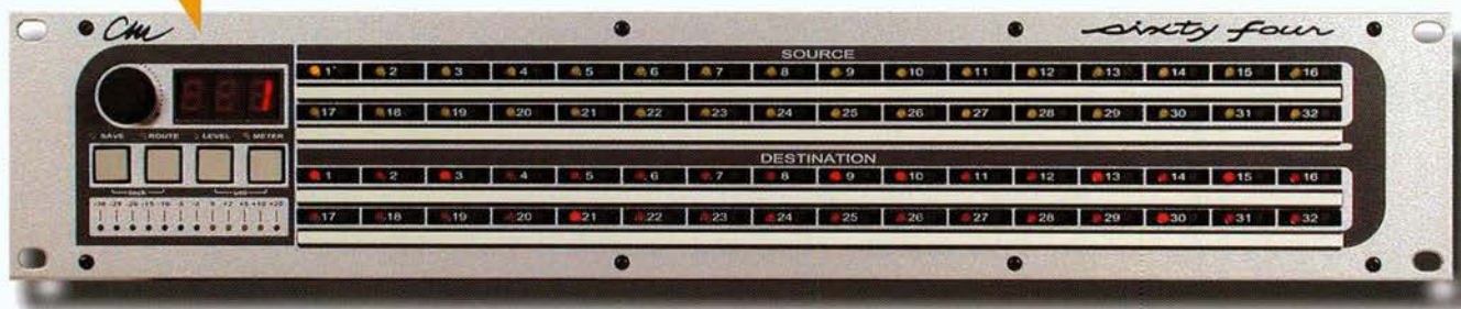
MULTIPLE UNITS CAN BE DAISY-CHAINED FOR PATCH CONTROL VIA MIDI OR THE RS-232 CONNECTOR.
