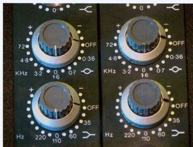
FIG. 1. THE FRONT PANELS ON THE TWO UNITS ARE SO NEARLY IDENTICAL THAT YOU HAVE TO KNOW WHERE TO LOOK TO TELL THEM APART. NEW ON THE LEFT AND OLD ON THE RIGHT.
