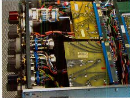
FIG. 3. THE IDENTICAL TRACES ARE ATTRIBUTABLE TO USING THE ORIGINAL PCB ARTWORK FROM THE NEVE ARCHIVES. NEW (LEFT) AND OLD (RIGHT).
