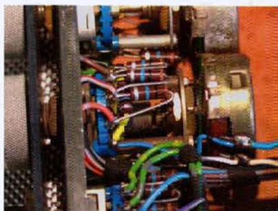
FIG. 5. COMPARE THE NEW METAL FILM RESISTORS AND SMALL POTS (TOP) WITH THE OLC BROWN RESISTORS AND CARBON POTS (EOTTCM).
