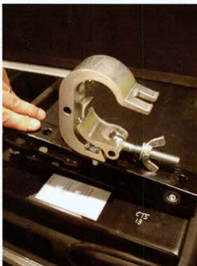
Vari*Lite hook bar snaps on. Means you can leave it on the truss, so the mover gets rigged in exactly the same place each time.
