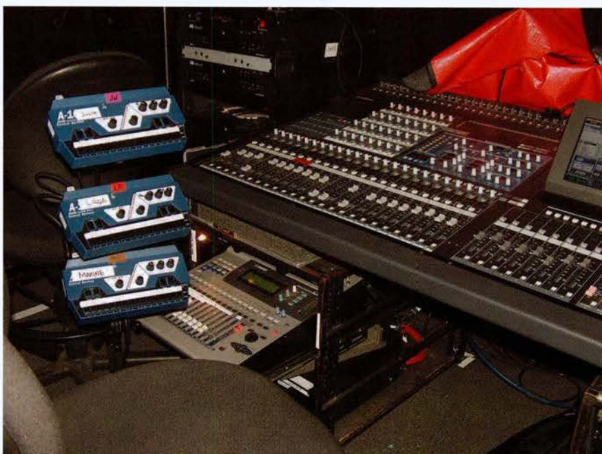
Monitor desk (PM5D) with a bunch of Aviom units and a Yamaha submixer underneath.
