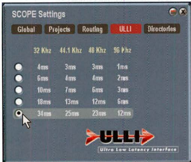
Fig. 2: When mixing, 20 or 30ms of latency will let you run more plug-ins, with a negligible tradeoff in performance.
