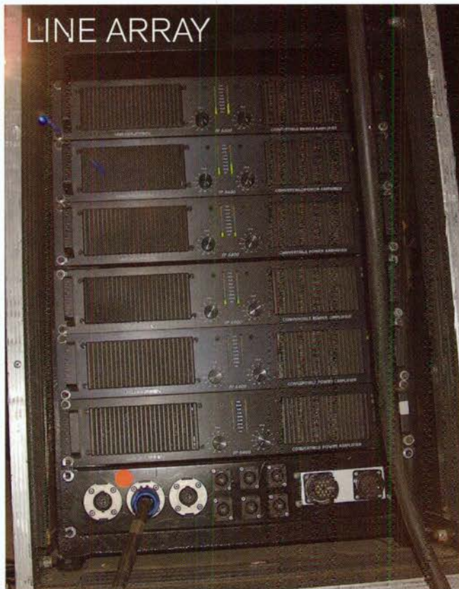
Lab Gruppen fp6400 amplifiers on hand to power the EAW KF-730's (and subs)
