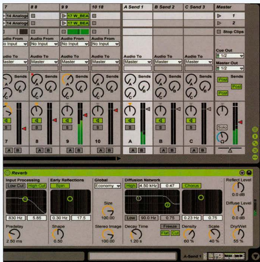
Fig. 1: Ableton Live's Reverb has been inserted into the A Send 1 bus, thus saving considerable CPU power over inserting several instances into multiple tracks.
