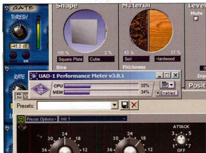
Fig. 3: Even running a reverb, heavy-duty guitar amp simulator, and limiter, the UAD-1 is using only 35% of its onboard CPU's capacity.
