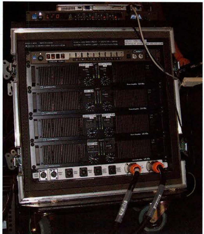
Kudo rack, LA48A amplifiers, Lake Contour (in rack) and Lake MESA EC (top)
