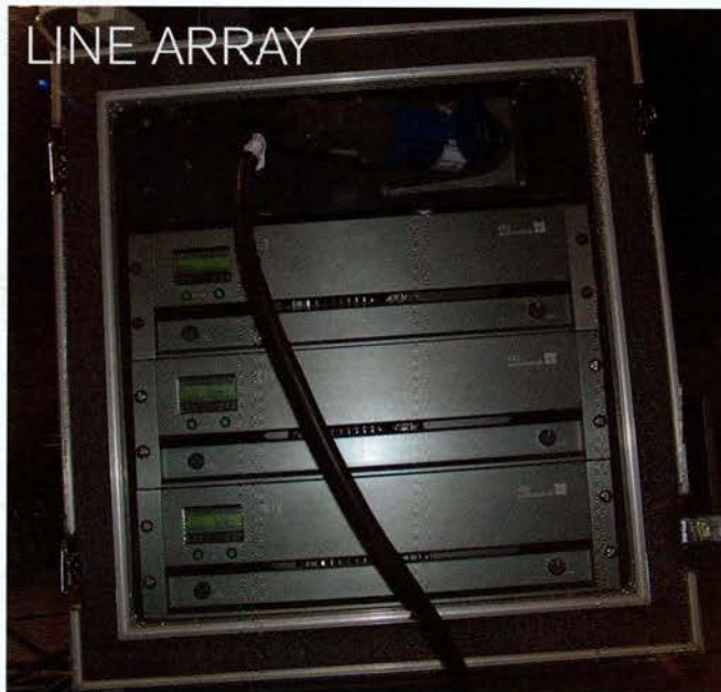
c+b D12 amps, internal processing
