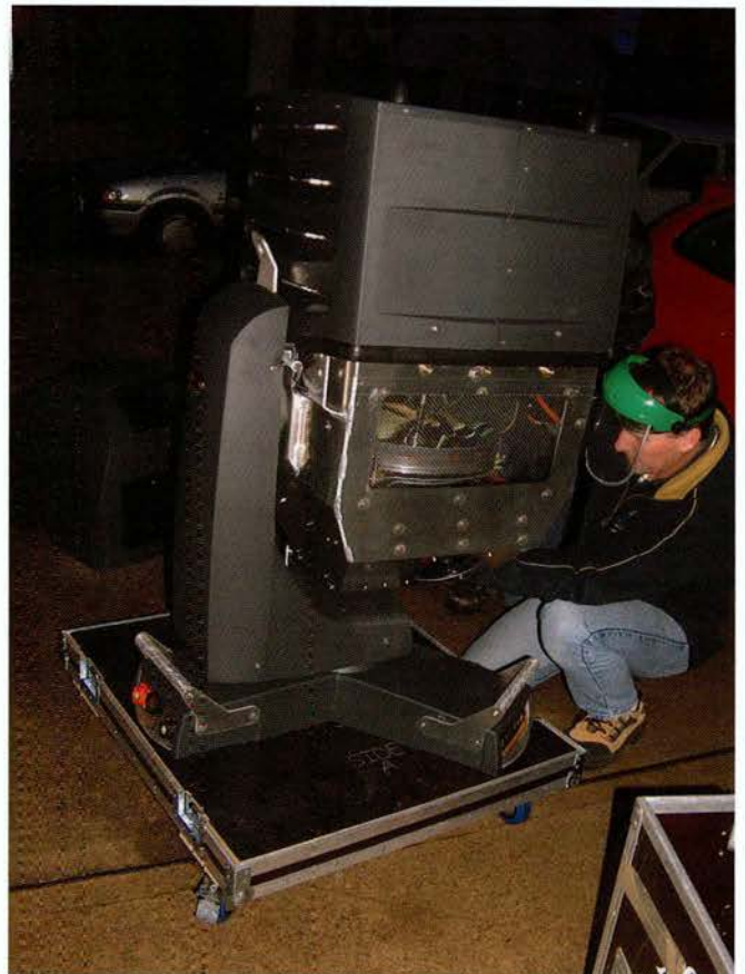
Gen Williams installs the lamp. A 4.5k xenon lamp needs to be handled carefully
