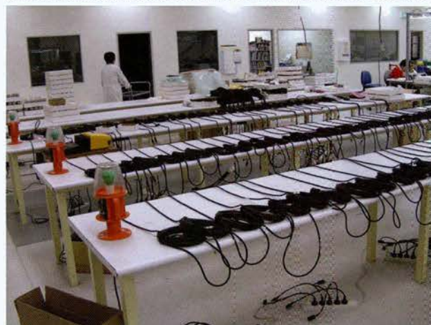
Test bench for a day's microphone batch (left). Valves are soak tested (right). Rode make almost everything in Sydney.
