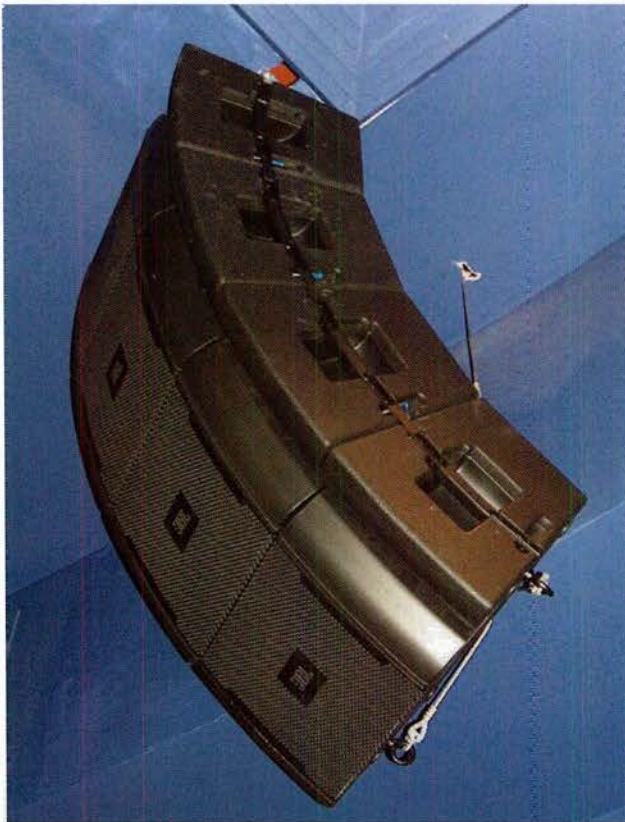
Vertical integral rigging flyware allows a vertical array of up to six boxes. In addition, one or two boxes can be stand (pole) mounted. Four boxes can be ground stacked and pointed upwards, to cover stadium seating from a playing field.
