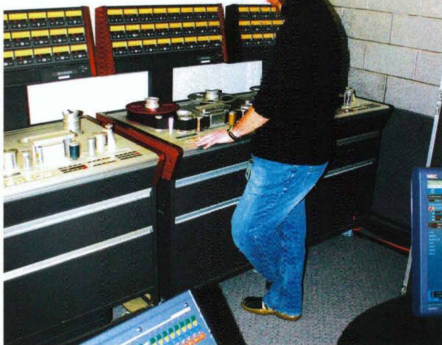
A spare for the spare. Technician Heath Conditte transfers material from one of Xepa's three Studer A827 machines.
