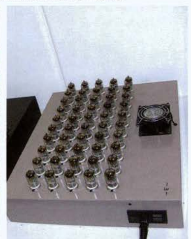
Test bench for a day's microphone batch (left). Valves are soak tested (right). Rode make almost everything in Sydney.
