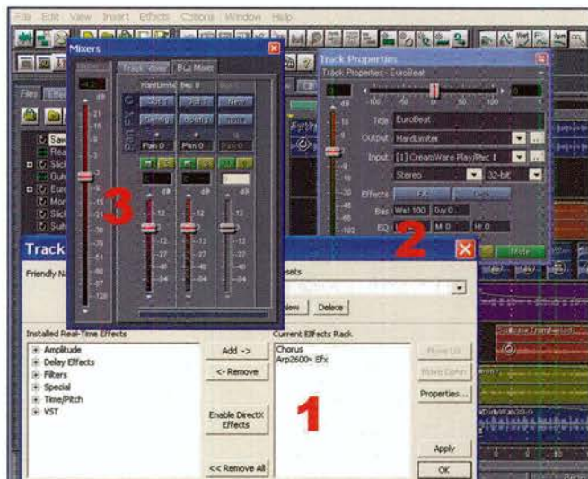
Fig. 2: Adobe Audition can add not only effects, but "effects racks" (1) into tracks or buses. Note that the tracks let you choose a wet/dry amount (2) for sending into buses, which are brought together in a separate bus mixer (3). As with Sonar, there's no "master effects" slot per se, because any bus can serve as a master bus, and include effects.
