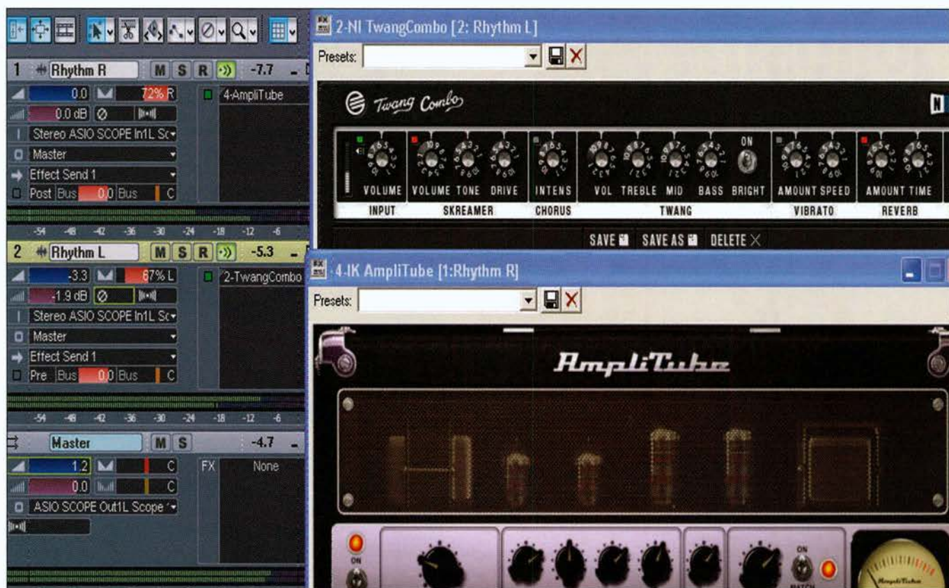
Fig. 1: Native Instruments' Twang Combo and IK Multimedia's AmpliTube 2 are being treated like a guitar setup that splits into two different amps. Each plug-in is inserted into its own track, but fed by the same guitar signal.
