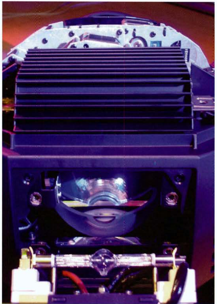
The Mac 2000 inspired lampgate has been moved for easier access
