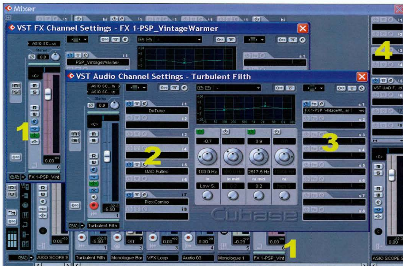
Fig. 1: With Steinberg's Cubase SX3, insert, send, and master effects all have six pre-fader and two post-fader slots, and look similar. Send effects go in a separate FX track (1), which returns to the mixer. Individual channels have inserts (2), as well as eight send controls (3). The master outs (4) have a similar structure.
