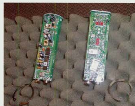
Fake circuits appear hand soldered.
