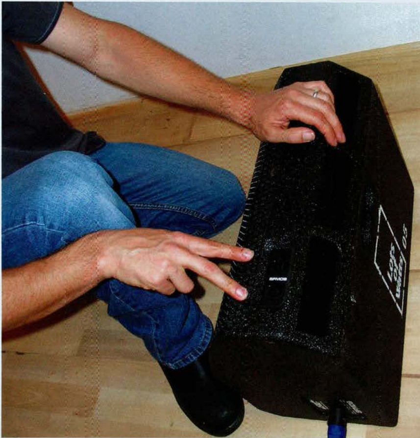
The SFM has three pairs of Speakon connectors for near invisible wiring - one pair each side, and one pair under the front.
