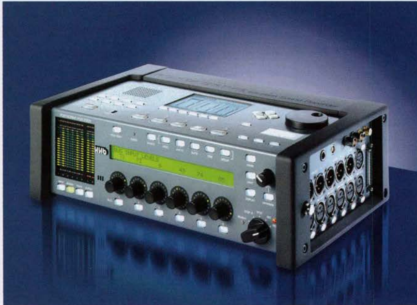
HHB Portadrive 8-channel 24-bit 96kHz on removable 40GB HD.
