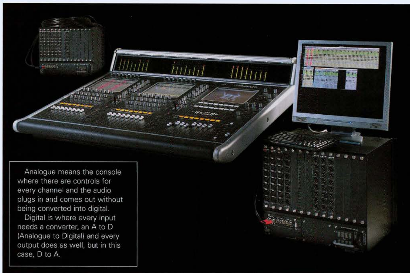
Digico D1. Same performance as a D5, but with less control surface.
