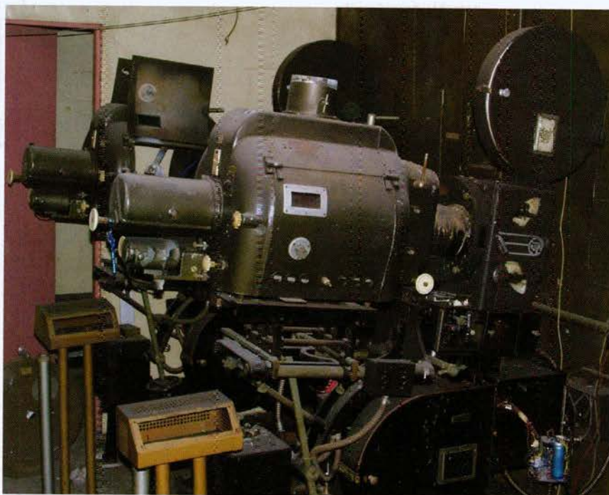
Open arc projectors dating from 1927 were still in place.
