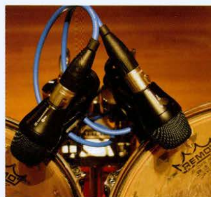
Rack toms miked with dynamics. Note the positioning to minimise spill
