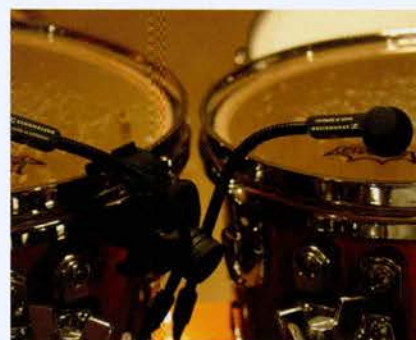
Gooseneck condensers used on rack toms
