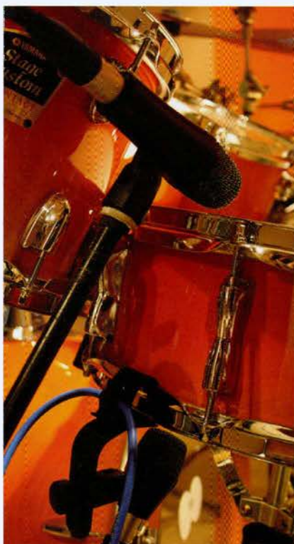
Double miking can tighten up a dull sounding snare
