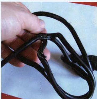
It doesn't look so good when you undo the cable tie.
