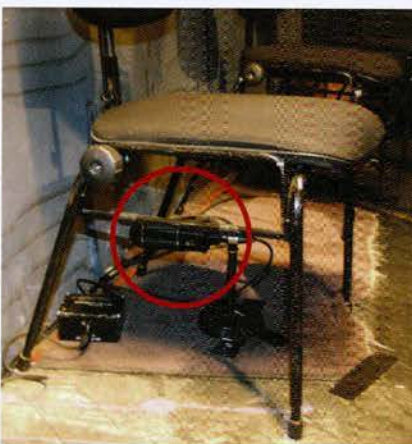
Innovative microphone techniques no. 1 - Ribbon mic under a chair for the french horns.
