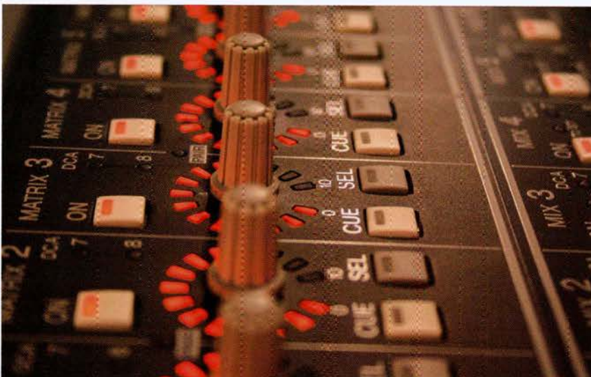
You could even use the matrix outputs as submixes for multitrack if you're short of tracks.
