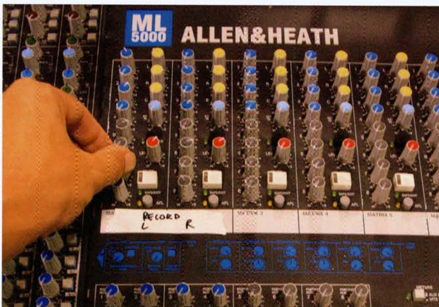
Using the matrix for recording allows the operator to make adjustments to the record mix without messing up the live show.
