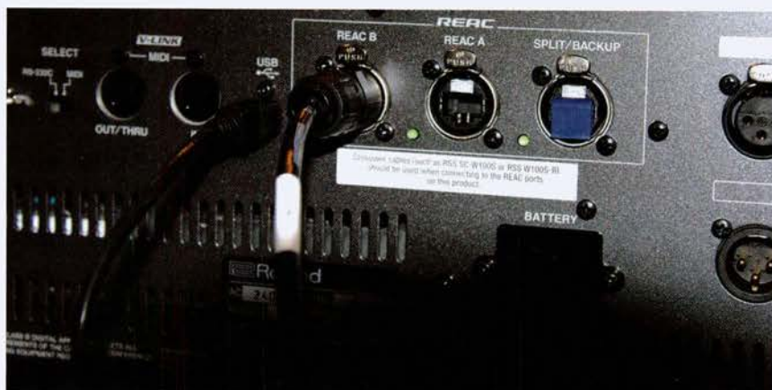
REAC inputs - this connection plus power is enough to make the system work
