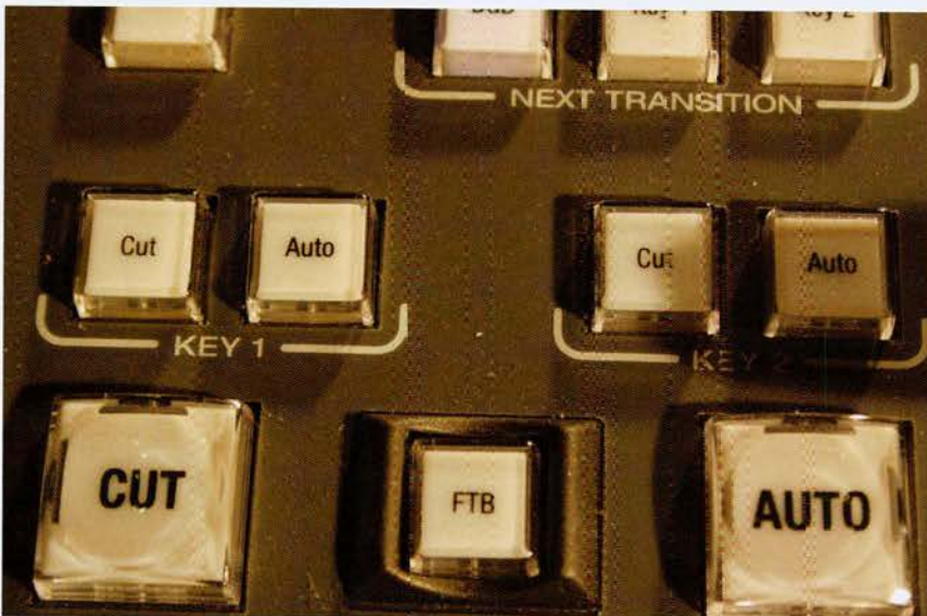
Note the nice little protector around the FTB switch - good attention to detail!
