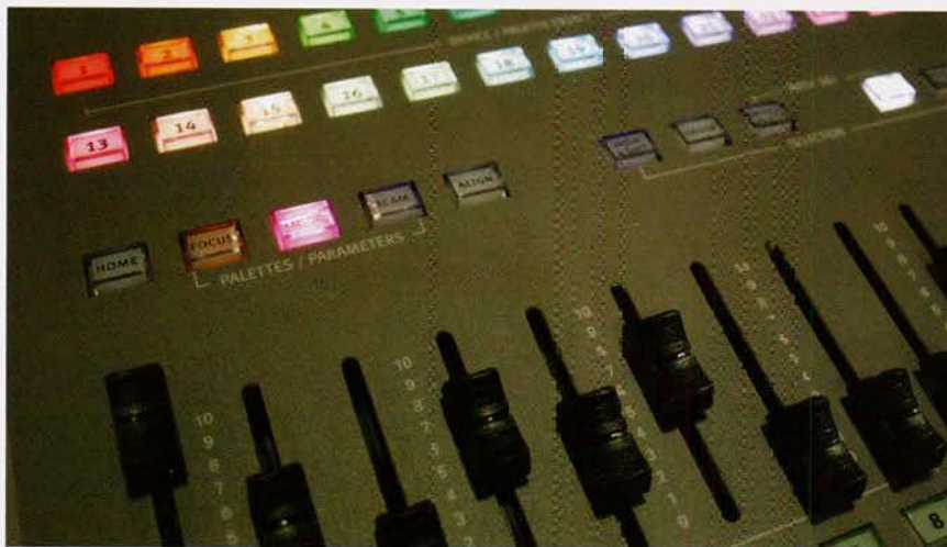
The colour mixing LEDs preview the palette colour for colour mixing fixtures
