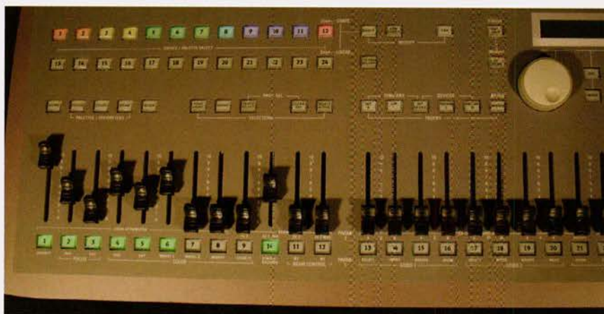
Control parameters are mapped to the faders. Green buttons indicate parameters available on this particular fixture
