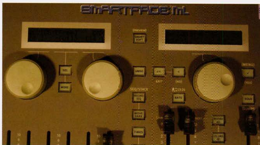
If you don't like using the faders, the encoders can be used to control fixtures. They also provide access to menu and patching operations.
