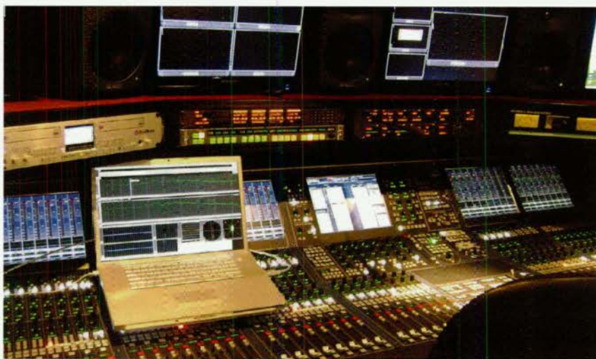
Inside ZerO1zerO's new HD truck: The Riedel's Artist Digital Matrix Intercom is seamlessly integrated with Lawo's Mc66 audio console & routing environment via Riedel's MADI client cards.
