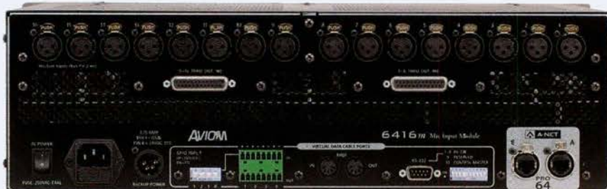
The back of the mic input box. Note the facility for a redundant PSU and the loop outs.
