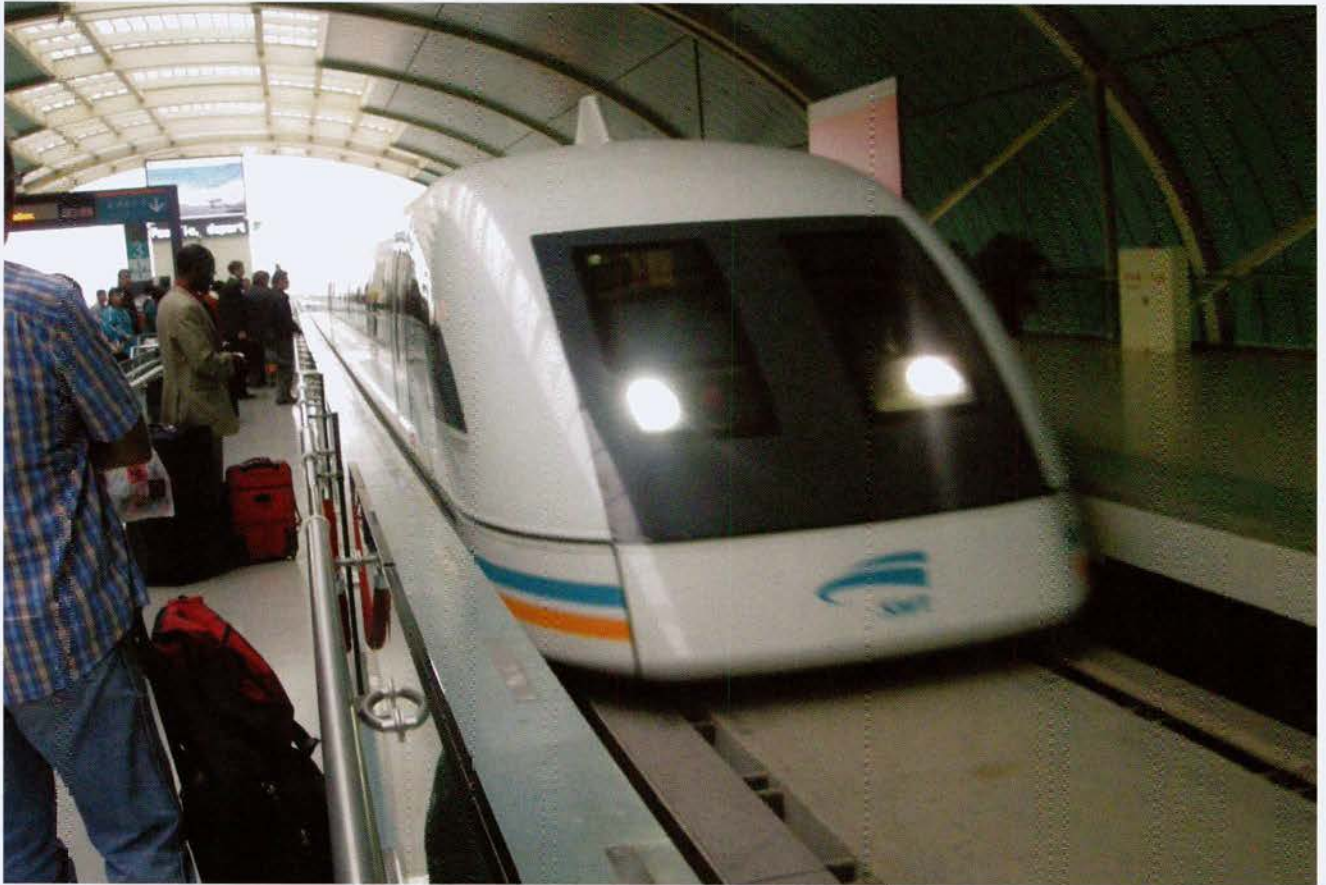
Maglev. Mindblowing futuristic Magnetic Levitation train that runs to Shanghai airport. Top speed 581 kmh, best it would do for CX was just 370 kmh.
