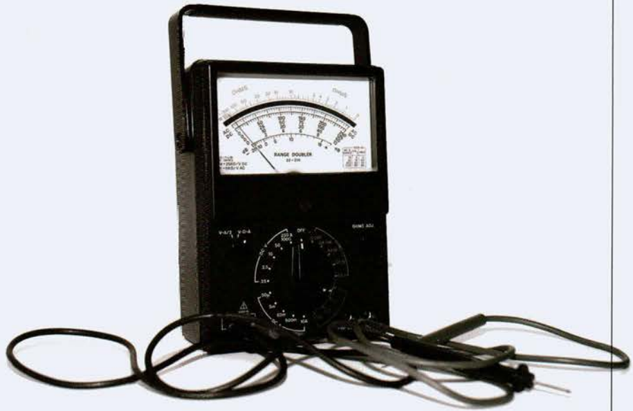
Ohmmeter – all well and good for resistance, not so flash on impedance.
