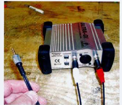
One i-Pod (or PC) stereo feed into a single DI or channel is: Not How We Do Things! Use two DI's or 2 console channels.
