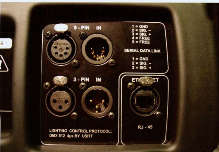
3 pin, 5 pin, and RJ45 connections
