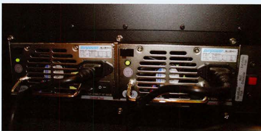
Dual redundant hot-swappable power supplies.
