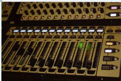
Faders are in banks of 12 with layer and page keys to the right.
