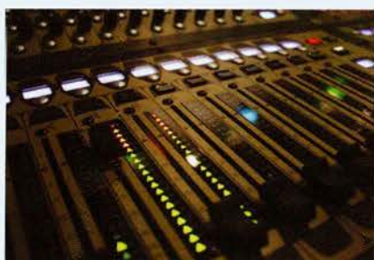
Channel strips have metering adjacent to faders.
