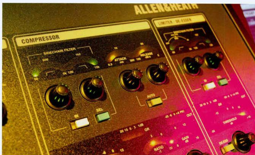
Auto timing on compressor.
