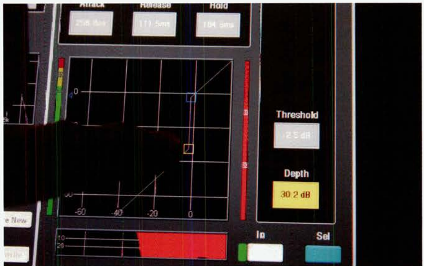
As well as using the rotaries, you can change some parameters by dragging on the touch screen.
