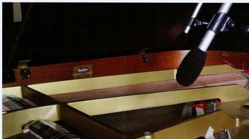
Moving the mic over the bass strings further from the action offers more low frequency response.
