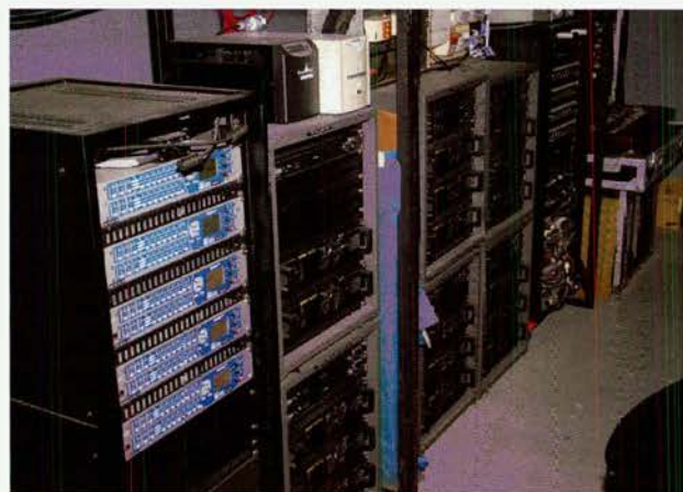
Five Galileo processors and racks of Yamaha amps (for all the MM4s). The DM2000 on the end handles foldback.
