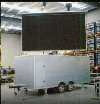
13sqm Lighthouse mobile LED Screen, 16mm resolution
