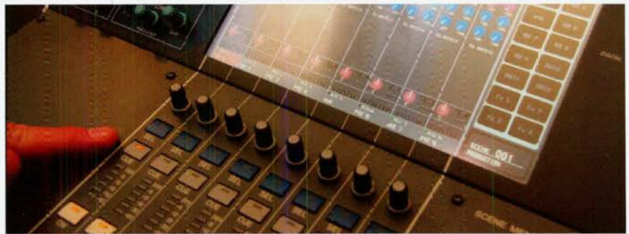
Send on fader mode, cue bus sends mix 1 to listen wedge.
