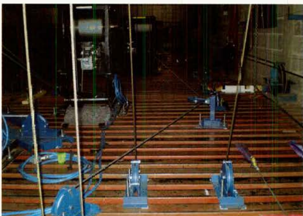
Winches and diverted lines atop grid.
