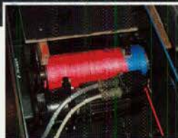
Winches with the kevlar based rope. No tools required to re-tension the trucks!
