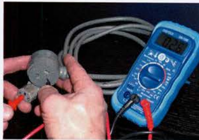
NOT the way to test for Earth Resistance....
