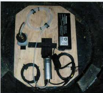
Gotta love the gadgets - above is the inside of a prop "pot of stew". The little smoke machine is the silver tube in the centre, the smoke fluid is on the left and an older style camera battery on the right. An actor simply pushes an external button, and smoke is created with no pre-heat time! This little guy is not cheap, but it is now in the hire inventory of Chameleon once this tour ends.
